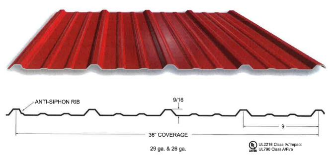
Flat-Loc -- a low profile, stout-ribbed panel ideally suited for roofing or post-frame buildings. Manufactured in 29 ga., 26 ga., and 24 ga. Minimum recommended slope is 3:12 with sealant.
