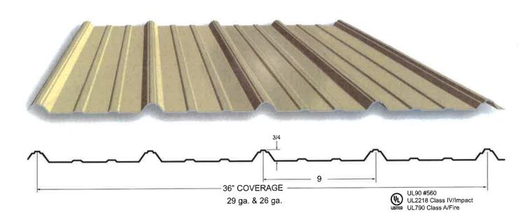
AG Panel - a low-profile, economical panel solution for residential, commercial and agricultural roofing or post frame buildings. AG panels are a very durable, high-value metal roofing system. Manufactured in 29 ga., 26 ga., and 24 ga. Minimum recommended slope is 3:12.
